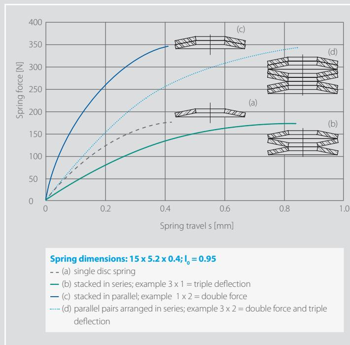
If disc springs of different thickness are stacked in a suitable way, then even progressive characteristic curves can be realized. For this, either several disc springs of different material thickness or identical disc springs with intermediate rings of different thickness or different layering types are used.
