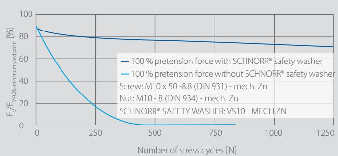
Extensive test series carried out at independent public material research laboratories prove that the original SCHNORR® safety washer brings about a clear improvement of the safety properties
